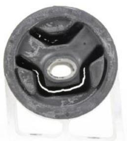
Figure 2 - The engine mount
