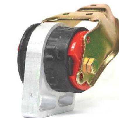
Figure 4 - showing polyurethane insert fitted inside the engine mount
