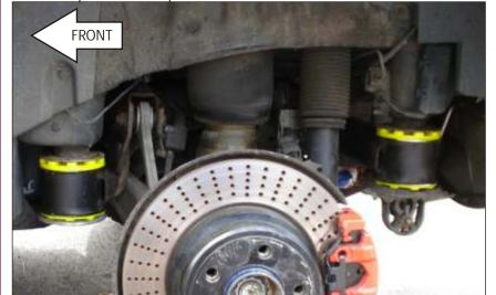
Fig 3. Front and rear mount - complete assembly.
