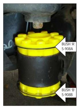
Fig 1. Front mount - partial bush fitment.
