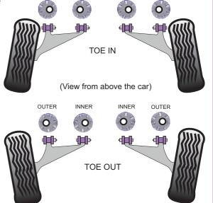
Hole positions in the sleeves, looking at them from the outside of the car on both sides, showing maximum adjustment limits. The adjusters will have to be adjusted individually to achieve the desired toe and camber settings.
