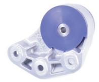
Align B bush with cast features on bracket
