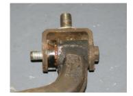
PFR17-207W fitted in the same way as PFF17-201 with top-hat section installed towards centre of wishbone. Note washer locations.
