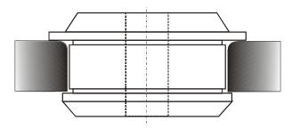
Ensure large diameter of polyurethane bush is located to towards the side of the arm with a radius.
