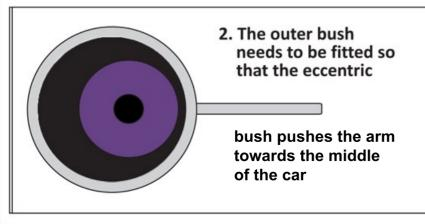
3. Please reset steering geometry after fitting any new suspension bushes
